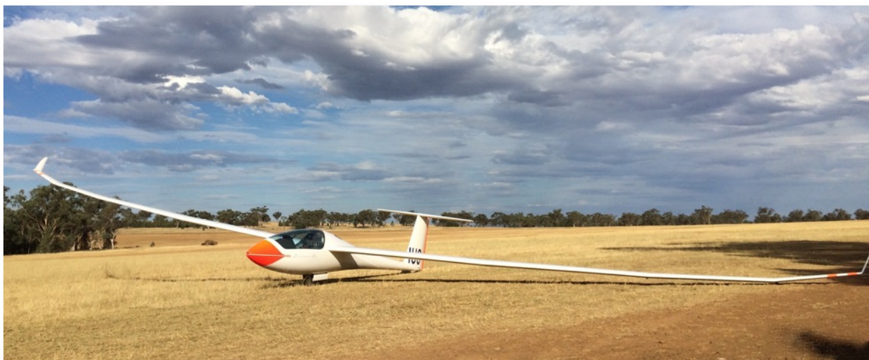
On the Southern Cross short list: a Discus 2c with 15/18 metre span. This one was pictured at Lake Keepit.
