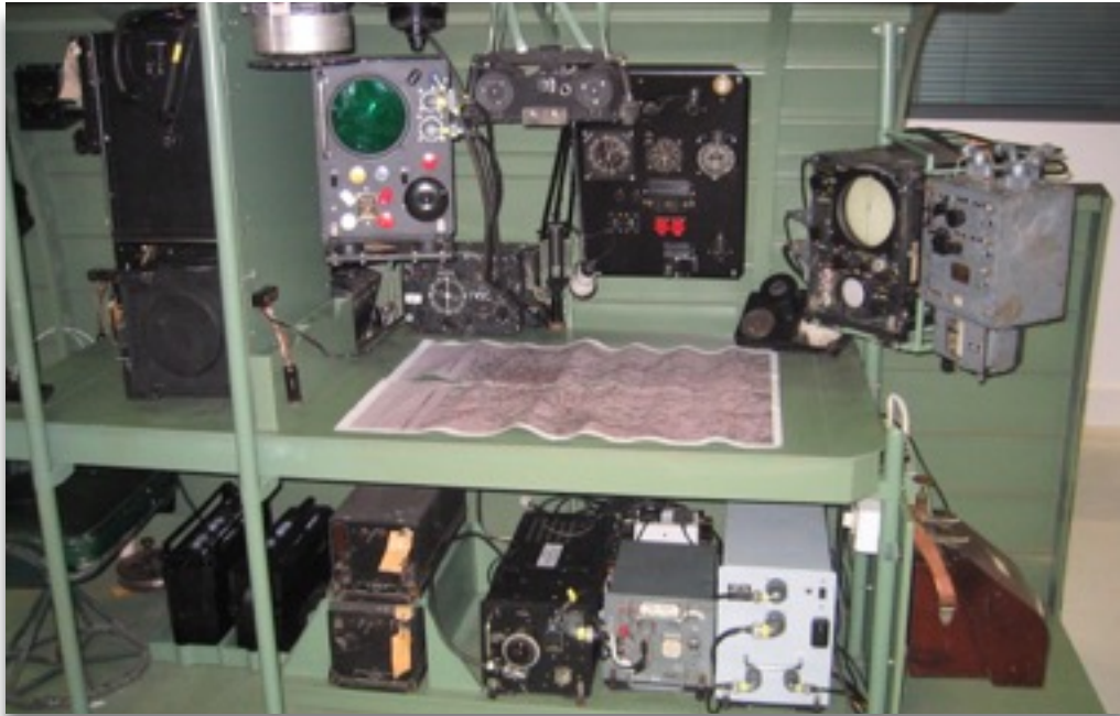
Lancaster Navigator's table with Gee indicator at the left and the H2S radar Plan Position Indicator and its controller at the right. The receivers and power supplies are under the table in this full-size replica built by the Duxford Aviation Society.
